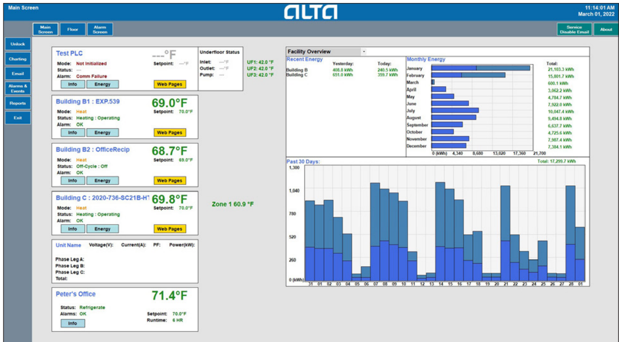
Figure 5. ALTA's central HMI aggregates data from across its installed base of EXPERT systems.
