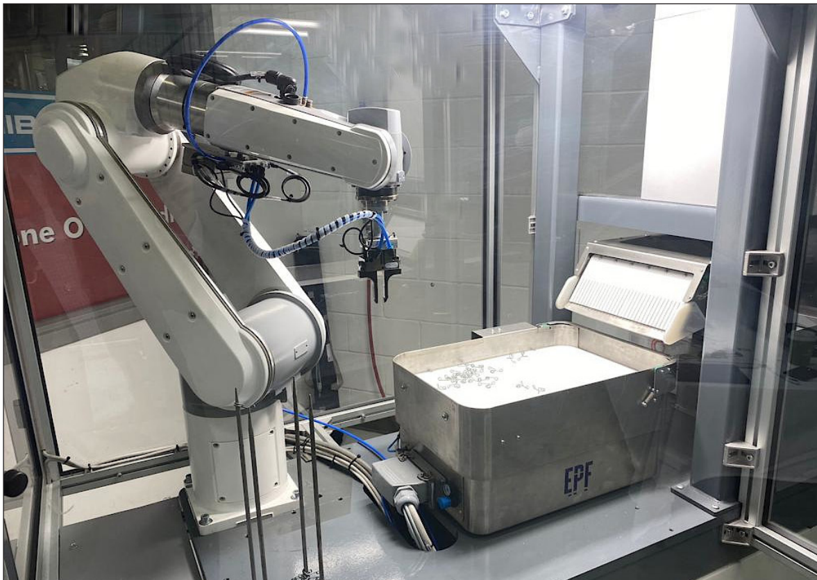
Figure 1. The Supata system consists of feeding, vision, and robotic handling systems, and a control system/human-machine interface (HMI).
