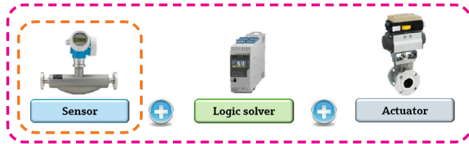
Option 1: Functional test of the entire SIS Option 2: Partial testing of the SIS
