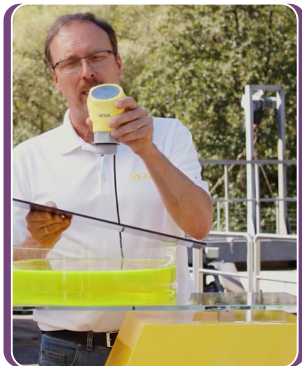
Jürgen Skowaisa demonstrates how a radar sensor can measure level through the plastic material of a typical container.
