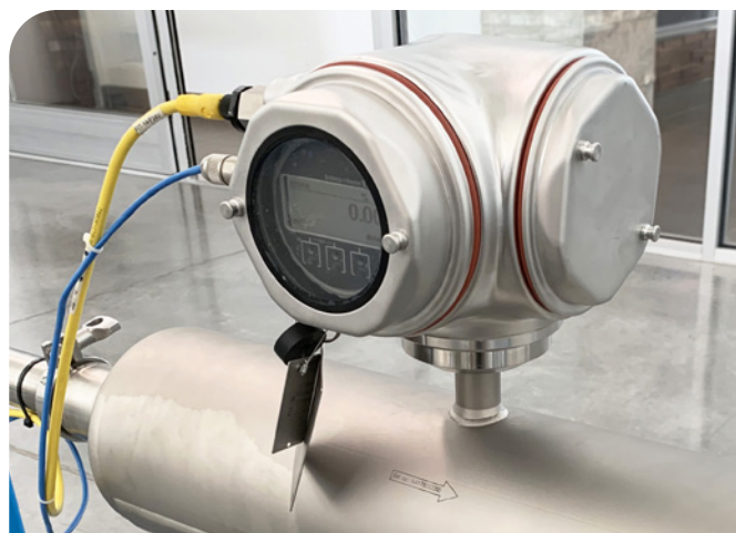
Figure 2. A Coriolis flowmeter, such as this Endress+Hauser Promass, makes multiple measurements that can be used for inline quality control.
