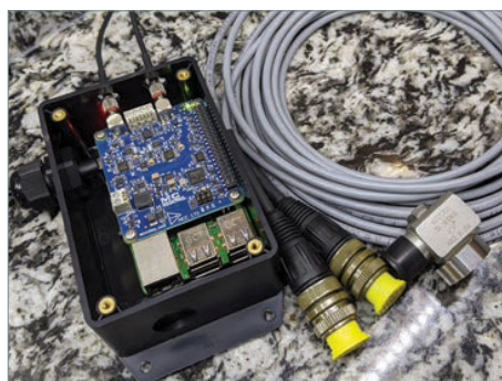
The MCC DAQ HATs fit easily within the existing system enclosure.
