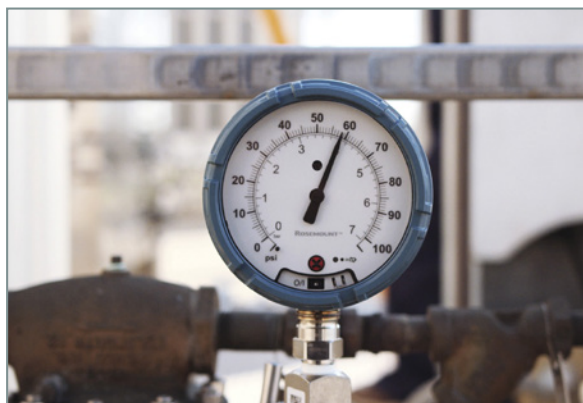
Figure 6. The Rosemount Wireless Pressure Gauge and Smart Pressure Gauge are identical except for the wireless capability.
