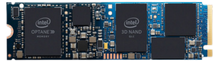
Figure 2. M.2 Intel Optane Memory: Intel's speed-boosting cache storage in an M.2 format. Developed to accelerate cache for another drive to enable high-speed computing
