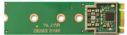
Figure 4. M.2 TPU: Tensor Processing Unit, developed by Google to accelerate training on large and complex neural network models. A powerful and energy-efficient AI accelerator in a compact M.2 form factor.
