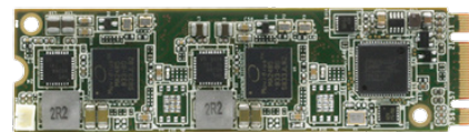
Figure 3. M.2 VPU: Intel's Movidius VPU (vision processing unit), developed to enhance machine learning and inferencing for edge computer vision that requires robust and compact technologies.
