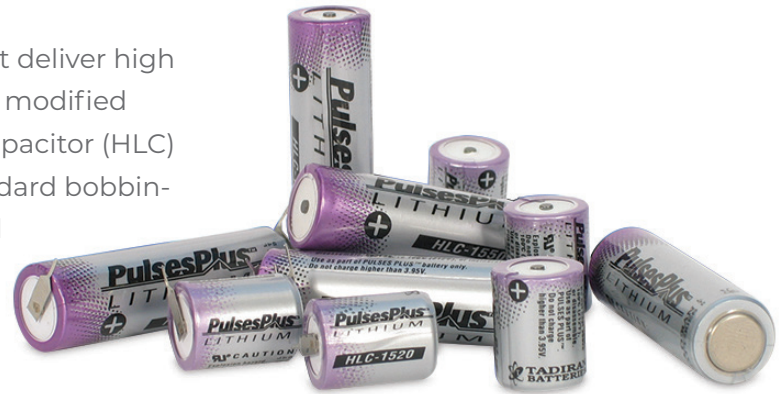
Figure 6. Bobbin-type \text{LiSOCl}_2 batteries can be combined with a patented hybrid layer capacitor (HLC) to offer up to 40-year operating life while providing high pulses to power two-way wireless communications.
