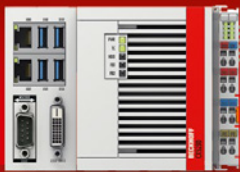
CX5230: Intel Atom® x5-E3930, 1.3 GHz, 2 cores
