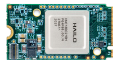
Figure 5. M.2 Hailo-8: AI Acceleration module—a best in class inference processor packaged in a module for AI applications; offers 26 tera operations per second and compatibility with NGFF M.2 form factor, M, B+M, and A+E keys.
