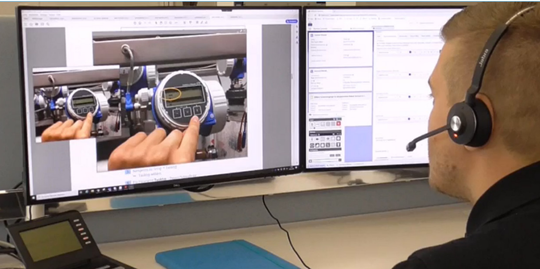
Figure 1. Using an augmented reality application, support engineers can see everything the technician sees in the field, and then guide troubleshooting or maintenance efforts using a virtual pencil to highlight target components for the technician.
