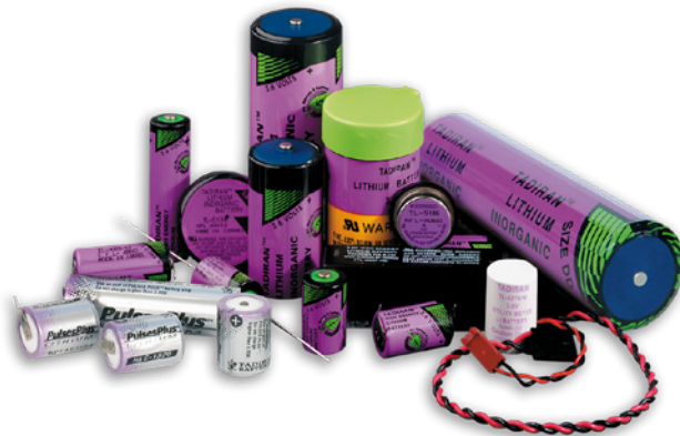
Figure 2. Bobbin-type LiSOCl 2 batteries are preferred for remote wireless applications, delivering high energy density, up to 40-year service life, and the widest possible temperature range, making them ideal for use in inaccessible locations and extreme environments.
